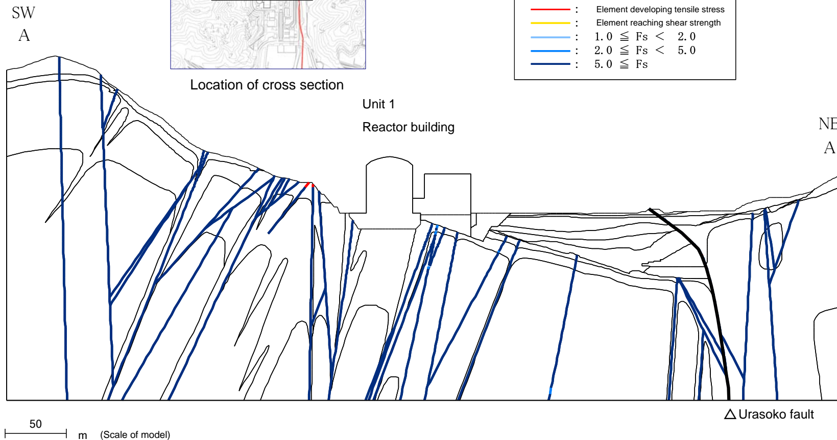
Fig. Distribution of local safety factor of shatter zones (cross section at Unit 1)
